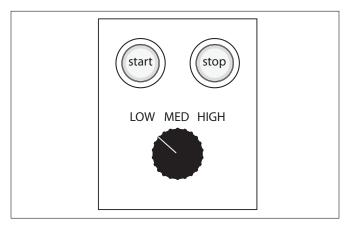
Located on top of the unit the mode buttons, with button LED lights. Low, Medium and High fan settings allow users to adjust the level of air circulation
